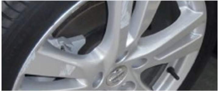
Major scuffing on wheel greater than 10% of surface area
