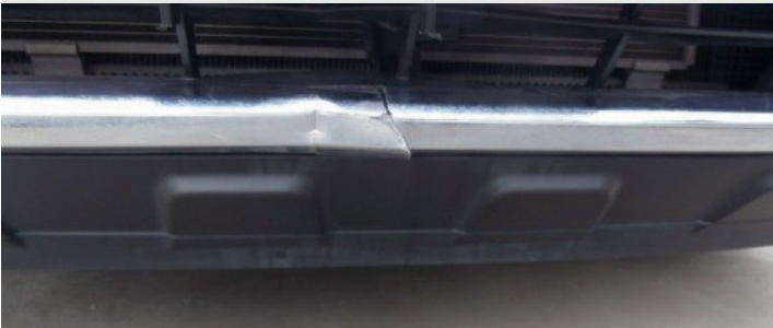
Cracked and dented bumper and grille
