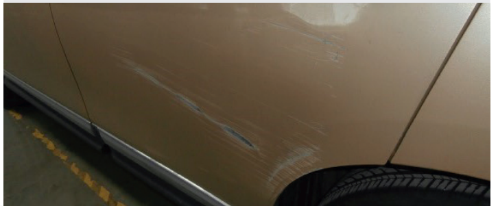
Scratches and abrasions greater than 40mm in length
