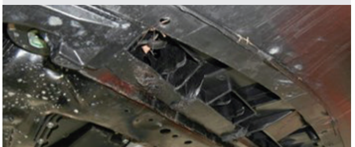
Deformation / major impact damage
