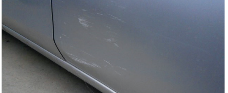
Scratches and abrasions greater than 40mm in length
